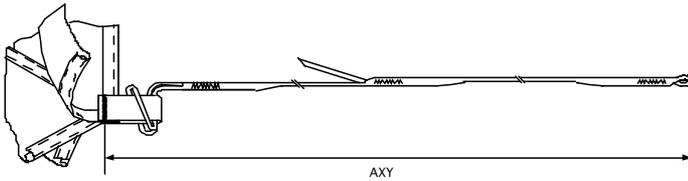
MEASURE FROM END OF SUSPENSION LINE LOOP TO BARTACK ON SUSPENSION LINE ATTACHMENT TAB.
